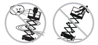
Do not drive the machine on or near uneven terrain, unstable surfaces or other hazardous conditions with the platform raised. Do not place or attach fixed or overhanging loads to any part of this machine.
