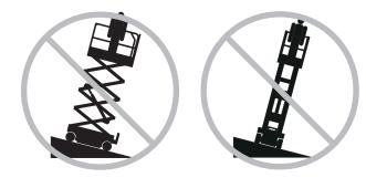
Do not depend on the tilt alarm as a level indicator. The tilt alarm sounds on the chassis and in the platform when the machine is on a severe slope.
